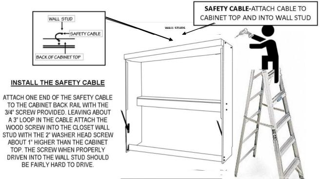
THE FUNCTION OF THE SAFETY CABLE IS TO MAKE ATTACHMENT FAILURE OF THE BED VISABLE BY ALLOWING THE BED TO COME AWAY FROM THE WALL 2 TO 3 INCHES. WHEN YOU SEE THIS CONDITION **DO NOT OPEN THE BED!** YOU MUST INVESTIGATE WHAT IS WRONG AND CORRECT IT!
