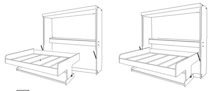
INSERT TRUNION BOLT Line up the trunion hole in the bed tray with the connecting threaded hole at the upper end of the lever arm bracket mounted to the cabinet side panel. From behind the unit, slide the trunion sleeve and bolt through the hole in the lever arm bracket. Once both trunions are in place, use the 10mm allen wrench to firmly tighten the trunion bolts.
