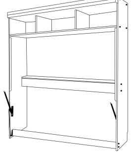
**ATTACH CABINET TO WALL** Be sure that the cabinet is perfectly square on the wall. Use the (6) 3/12" wood screws to attach the cabinet into 3 wood studs in the wall through the back of the top.
