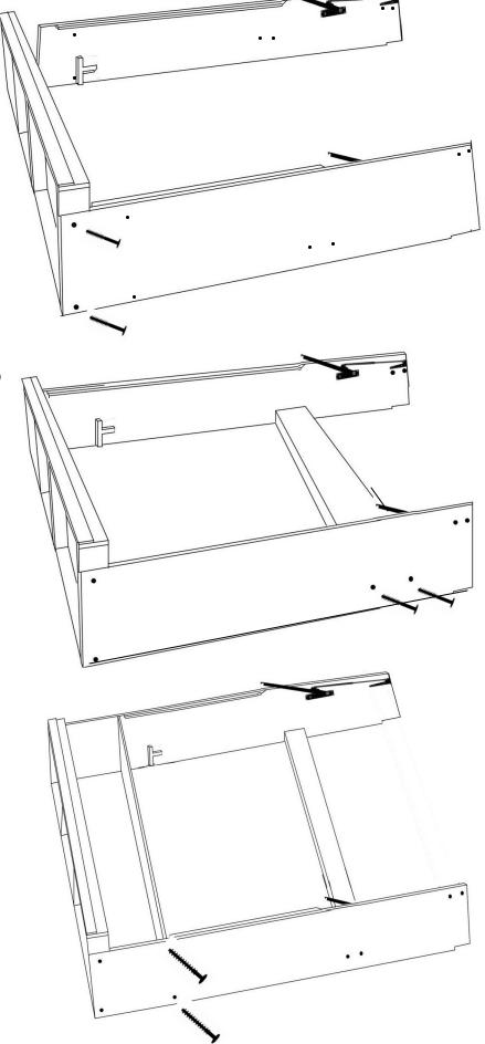
5 ATTACH LOWER STRONGBACK Insert lower strongback between the cabinet sides and attach with confirmat bolts (B) keeping finished edges to front.
