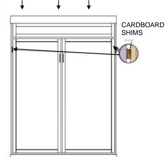
USING A STUD FINDER, LOCATE 3 WOOD WALL STUDS BEHIND THE BED AND MARK THEM WITH A VERTICAL LINE EXTENDING A FEW INCHES ABOVE AND BELOW THE CABINET TOP.WITH TWO PEOPLE TILT YOUR WALLBED INTO POSITION AGAINST THE WALL, MAKING SURE THAT ALL 3 STUD LINES ARE BETWEEN THE 2 SIDE PANELS. READCH OVER THE TOP OF THE UNIT AND DRIVE 6 -3 1/2" WOOD SCREWS THROUGH THE TOP ASSEMBLY BACK RAIL INTO THE WALL STUDS.
