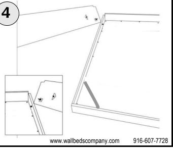
**MOUNT THE PISTONS BY FIRST SNAPPING** THE SHAFT END ONTO THE ADJUSTABLE BALL STUDS MOUNTED ON THE SIDE OF THE TRAY END. GRASP THE BARREL END OF THE PISTON AND ROTATE IT 180 DEGREES SO THE END SOCKET FACES THE BALL STUD ON THE TRIAN-GLE PLATE FOUND
