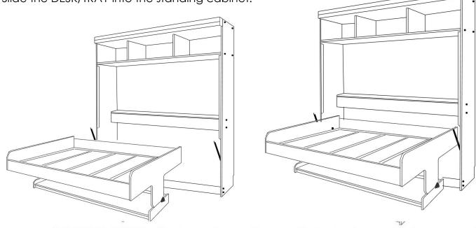
INSERT TRUNION BOLT Line up the trunion hole in the bed tray with the connecting threaded hole at the upper end of the lever arm bracket mounted to the cabinet side panel. From behind the unit, slide the trunion sleeve and bolt through the hole in the lever arm bracket. Once both trunions are in place, use the 10mm allen wrench to firmly tighten the trunion bolts.
